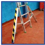
Folding stabilisers lock into position to provide secure positioning and stability.
