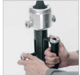
First, clamp on the long clamping jaw and then the short one. Then fully insert the long pins.
