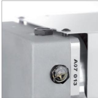
To vent the system stand pump unit upright and lower down clamping tool; operate tool several times without building up pressure.
