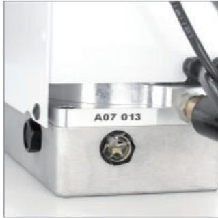
... or on its side (oil filler screw facing upwards). Do not overfill with oil.
