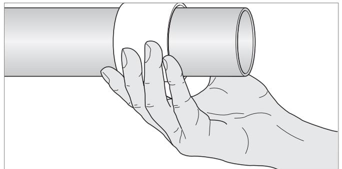
3. Expand pipe, rotate 30°, and repeat. The compression sleeve must not be in the expansion area. Expansion is to be carried out using the pressure switch or by activating the foot lever.
