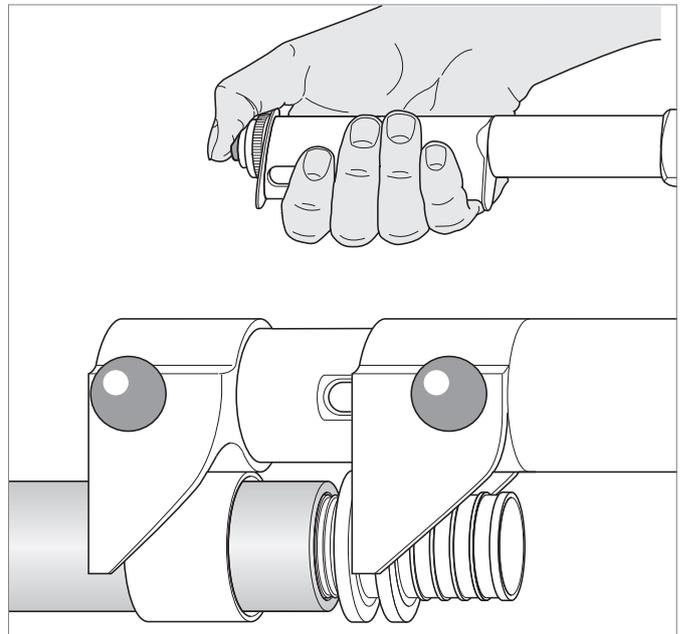
6. Insert the compression sleeve all the way up to the fitting collar by activating the pressure switch / foot lever.
