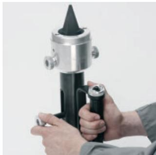
To exchange expander heads, remove fixing nut, position expander head correctly, screw fixing nut completely on. From dimension 75 mm, expander heads are screwed on directly (without fixing nut). Expander heads > 75 mm must also be screwed on completely. Avoid possible cants when mounting.
