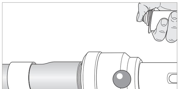
4. Insert fitting into pipe up to the stop. After a brief period the fitting will sit tightly in the pipe (memory effect).
