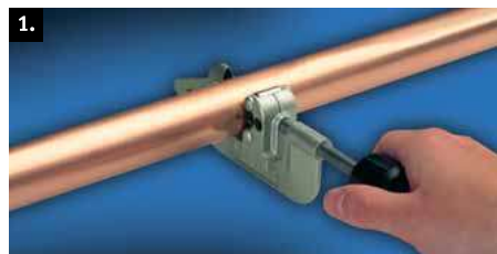
1. Cut the tube square using a rotary tube cutter.
