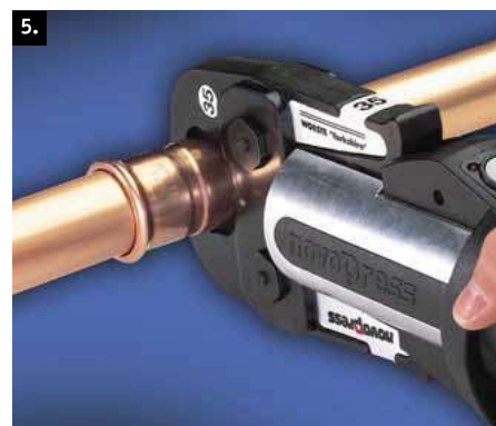
5. Press the trigger or button to start the jointing cycle. When the jaws fully enclose the mouth of the fitting, the joint is complete. The jaw should then be released from around the fitting.
