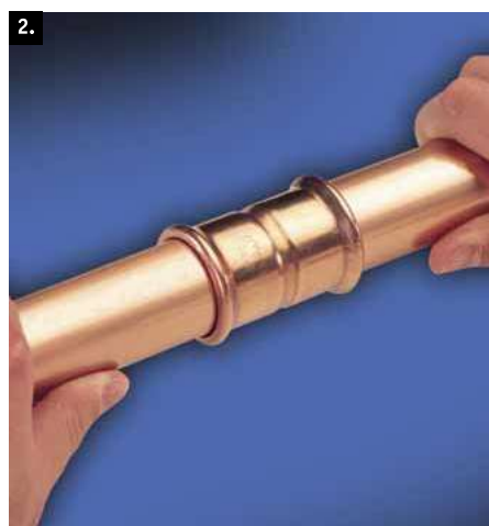
2. Assemble the joint, ensuring the tube is inserted into the fitting until it meets the tube stop, using the insertion depth mark as a visual aid. Only when the tube reaches the tube stop should the pressing operation be undertaken.
