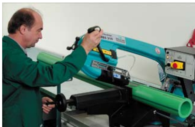
Before welding, the 160, 200 or 250 mm pipes are cut into the required lengths
