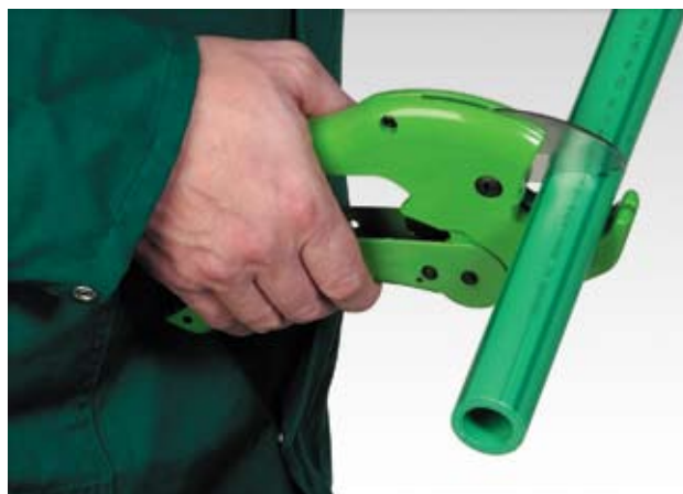
Cutting the pipe
