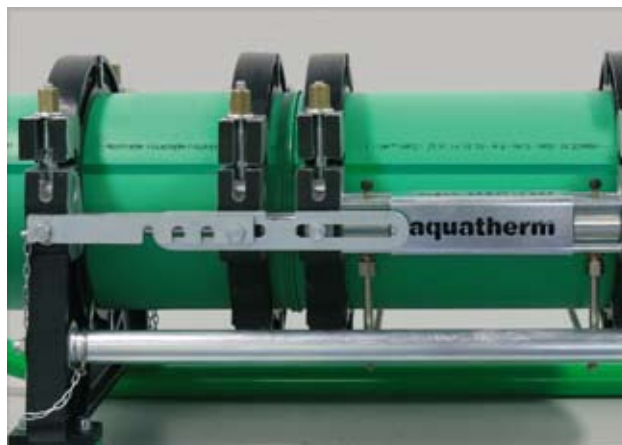
Join the pipes, cool down under pressure
