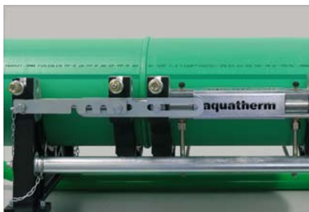
Unclamp and work on...
