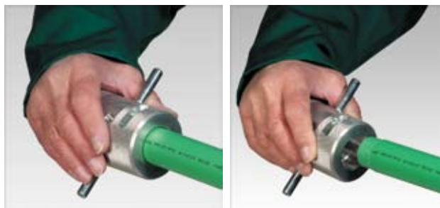
Peeling of the aluminium-PP-composite-layer
