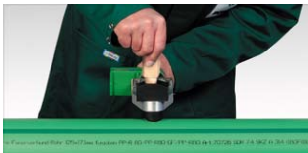
The welding tool is inserted into the pipe wall ...
