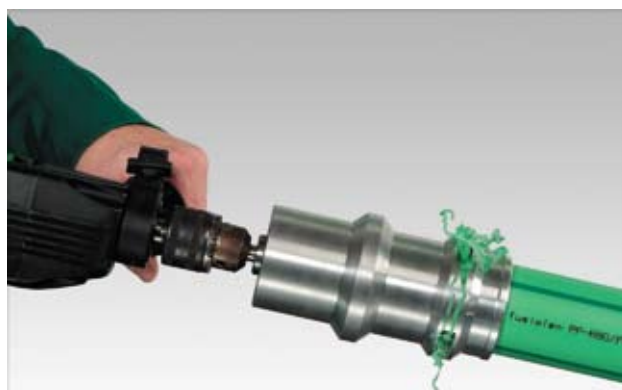
fusiotherm® peeling tool (Art.-No. 50558-70, up to 75 mm) (from 90-160 mm: Art.-No. 50572/50574/50576/ 50580 (without picture))
