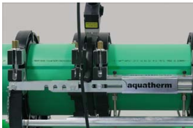
Positioning of heating element
