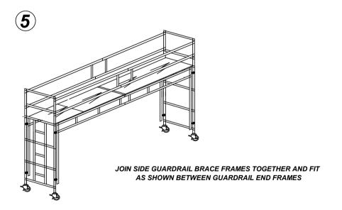
WHEN IN POSITION LOCK ALL CASTORS BEFORE USE FOLLOW ALL SAFETY PROCEDURES WHICH APPLY FOR THE SAFE USE OF SCAFFOLD TOWERS. WHEREVER POSSIBLE ALWAYS CLIMB UP THE INSIDE OF THE UNIT THROUGH THE HATCHDOOR. IF IN DOUBT DO NOT GUESS, CONSULT YOUR SUPPLIER.
