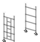
INSERT CASTORS AND ADJUSTABLE LEGS INTO END FRAMES, ENSURE LEG ADJUSTING NUTS ARE WOUND TO THE LOWEST POINT.
