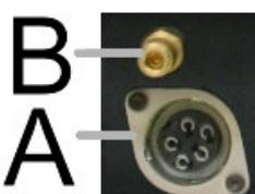
Finally, connect the gas hose from the TIG torch to the gas connector (B) on the front of the machine. If necessary, an extra gas connector for the fitting on the front of the machine is included in the package. Next, connect the fitting on the back of the machine to a gas regulator on the cylinder of gas to be used. An input gas line and the required fittings are also included in the package. Connect the TIG torch trigger to the trigger connector (A) on the front of the machine.
