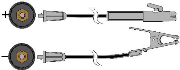
Connect the electrode cable to the (+) terminal and the work clamp to the (-) terminal. Insert the connector with the key lining up with the keyway and rotate approximately  $\frac{1}{4}$  turn clockwise. Do not over tighten.
