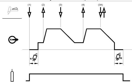
3. Press and hold the TIG torch trigger. The machine will now decrease the output current at a controlled rate, or downslope time, until the Crater current is reached.
