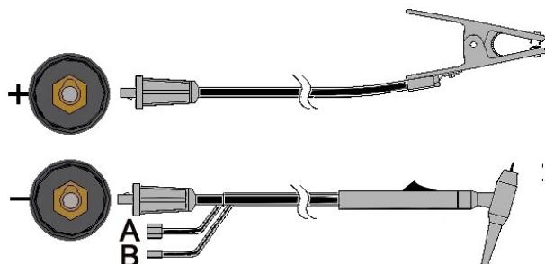
Connect the torch cable to the (-) terminal of the machine and the work clamp to the (+) terminal. Insert the connector with the key lining up with the keyway and rotate approximately  $\frac{1}{4}$  turn clockwise. Do not over tighten.
