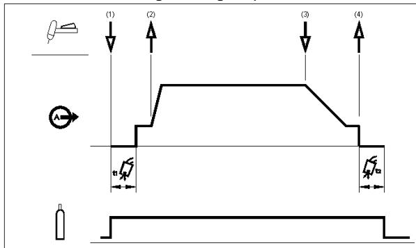
1. Press and hold the TIG torch trigger to start the sequence. The machine will open the gas valve to start the flow of the shielding gas. After the preflow time, to purge air from the torch hose, the output of the machine is turned ON. At this time the arc is started according to the selected welding mode. After the arc is started the output current will be at the Start current. This condition can be maintained as long as necessary.
