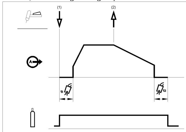
1. Press and hold the TIG torch trigger to start the sequence. The machine will open the gas valve to start the flow of the shielding gas. After the preflow time, to purge air from the torch hose, the output of the machine is turned ON. At this time the arc is started according to the selected welding mode. After the arc is started the output current will be increased at a controlled rate, or upslope time, until the Welding current is reached.
