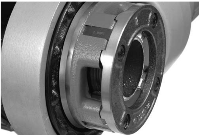
Figure 15 – Pipe Even with Edge of Dies
