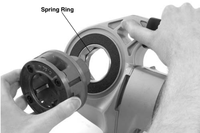
Figure 9 – Installing Die Heads into 600-I Power Drive
