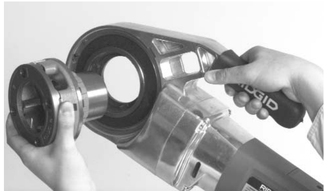
Figure 3 – Installing No. 11-R Die Heads
