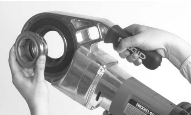
Figure 2 – Installation of 11-R Die Head Adapter
