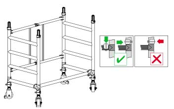
4 STEP 1: Connect two, 4 rung frames together.
