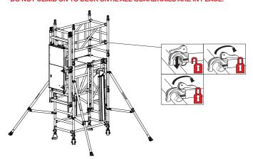
9 Standing up on the protected platform, lift the second trapdoor deck onto the platform. Store by the rear guardrail clear of the
