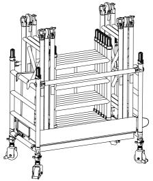
Add the final trapdoor deck in front of the 1m end frames. Fit the four SP4 stabilisers in front of the trapdoor deck. The trolley unit is now complete.
