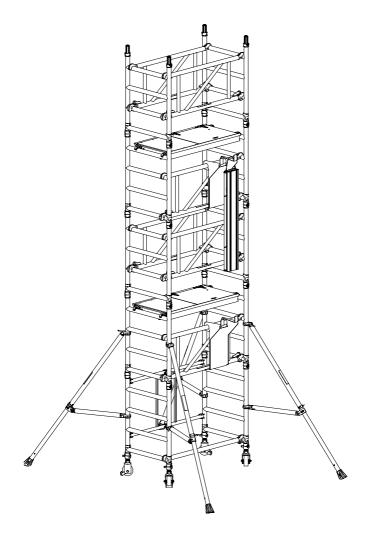
Unclip the storage strap from the folding toe board set, unfold and fit the toe board into position on the working platform. Move assembly brackets to base of the tower and fit to the lowest rungs of the end frames.
