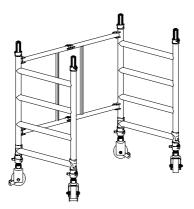
Locate the horizontal brace on the lowest rung with the hooks facing downwards - check the brace is correctly locked on the tube at both ends. Check the base unit is square and level using a spirit level. Adjust legs only to level and not to gain additional height.
