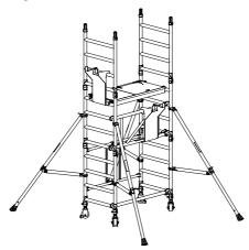
Hang four camlock guardrail units in order on the front assembly bracket and then 1 x folding toe board.
