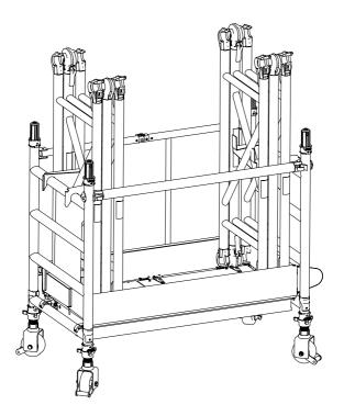
4 Place the 1m end frames in the centre of the trolley between the guardrail frames.
