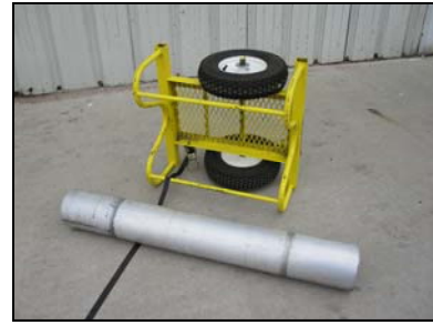
Place strap under pipe by rolling pipe.
