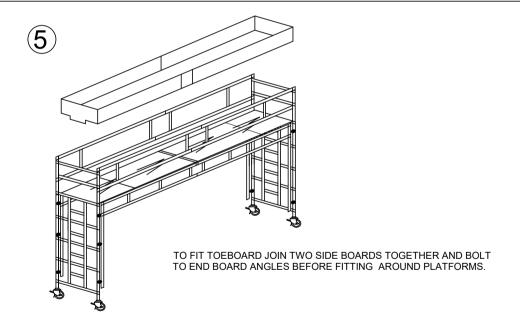
WHEN IN POSITION LOCK ALL CASTORS BEFORE USE FOLLOW ALL SAFETY PROCEDURES WHICH APPLY FOR THE SAFE USE OF SCAFFOLD TOWERS. WHEREVER POSSIBLE ALWAYS CLIMB UP THE INSIDE OF THE UNIT THROUGH THE HATCHDOOR. IF IN DOUBT DO NOT GUESS, CONSULT YOUR SUPPLIER.
