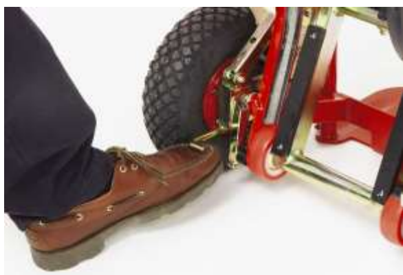
Switching the brake back to neutral position by foot or by hand.
