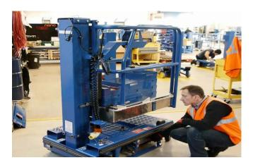
Apply an additional load to the platform, maximum 40 kilograms, so that the alarm and cut out operate.
