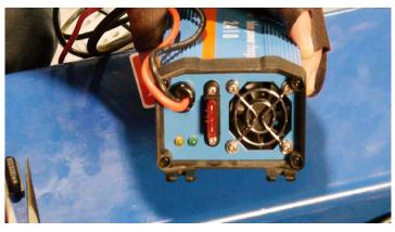
If there are no lights on the charger, check the supply connections which can be found on the right side of the chassis
