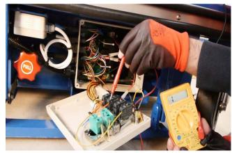
From the orange wires check the purple feed from the PCB, through the 'Suzi' cable and into the platform emergency stop switch at the control arm of the platform.
