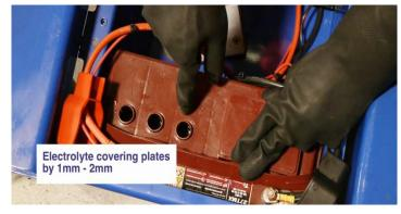
Check the connections and make sure the battery is clean
