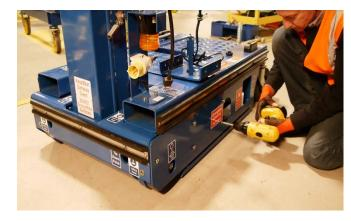
Remove the end buffer strip fixing bolts and bend back the buffer strip to reveal the M12 'c/sink' screw heads.
