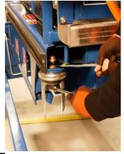
Refitting is a reverse of this procedure ensure it is torque to 55Nm. Ensure the wheel moves freely.
