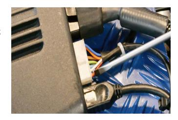
Using a continuity meter, follow the red wire into the ground enclosure and check the continuity.
