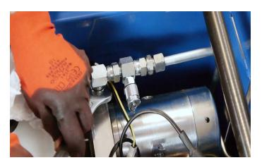
The new pipe is refitted in the reverse sequence. Ensure to connect both ends of the pipe loosely to ensure correct alignment and then tighten the cylinder connection first, taking care not to twist the pipe. It may be necessary to slacken the two power pack mounting screws located under the middle of the power pack to enable correct alignment. When
