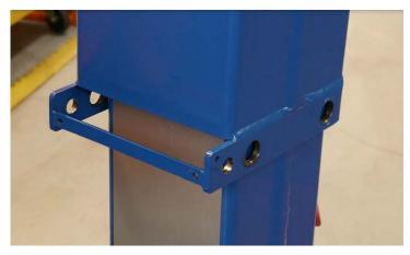
Repeat the process for the mast middle section. Access can now be gained for any maintenance or remedial work required. Reverse the procedure to reassemble the mast and platform. When reassembling the mast cap please ensure to apply a small amount of Loctite 648 to the locking bolts and torque to 30 Nm
