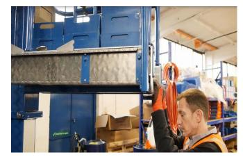
If the alarm does not operate, lower the platform and turn the adjuster screw anti clockwise until the alarm does operate, ideally with 20 to 25 kilograms additional force.
