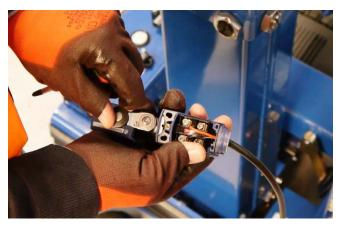
When checking the Hi/Low speed switch contact operation, depress the isolator switch. Failure to do so may lead to an ECU failure if a short circuit occurs
