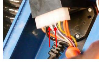
Then check from the switch to the timer module, and from the timer module, from the grey, through the 'Suzi' cable and back down to the PCB board. There will be a break in this circuit somewhere.
