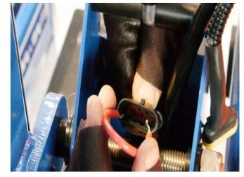
If the setting is OK, then check the switch plunger and connections by removing the tool tray and undo the four bolts and operate the lift function from the ground controls so that the mast caps complete with spring assembly, clears the mast section.
