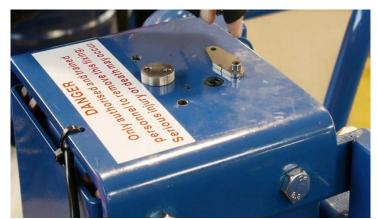
With the hoist, raise the mast outer section a short distance to a convenient position and remove the roller and wear screws. When removed lift the mast section clear of the mast using the hoist taking care to clear the inner stop blocks as the mast is raised.
