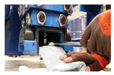
Locate the two power pack fixing screws, located under the base of the machine, below the centre of the power pack and undo.
