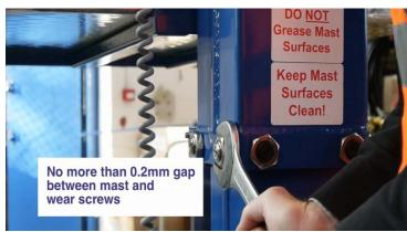
Adjust the two rear plastic wear screws in a similar manner. It is not possible to adjust the clearance between the inner and outer sections with the rear screws. Remove. Operate the lift function to ensure the outer and middle sections do not bind. Back off slightly any wear screws found to be pinching so that both mast sections travel up and down freely.
