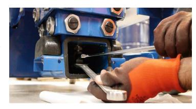
Check the Emergency lowering valve, spool and the valve screw cartridge on the side of the power pack.
