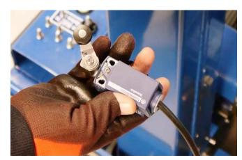
Using a continuity meter, check the two terminals and make sure the plunger makes and breaks the contact as the arm is moved. Note; the tilt override limit switch is located at the base of the mast below the flashing beacon. The Hi/Low speed switch is on the opposite side.
