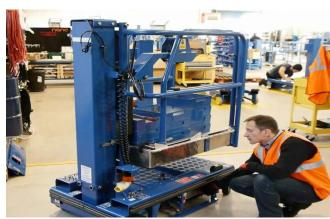
Apply an additional load to the platform, maximum 40 kilograms, so that the alarm and cut out operate.
