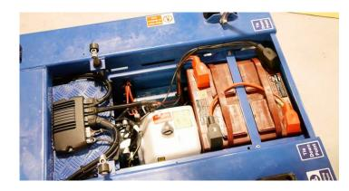
Check the electrolyte level in each of the battery cells.
