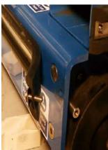
Place a suitable block under the ballast plate and undo the four M12 'c/sink' screws and slide the ballast block clear of the machine to reveal the spine and cap.
