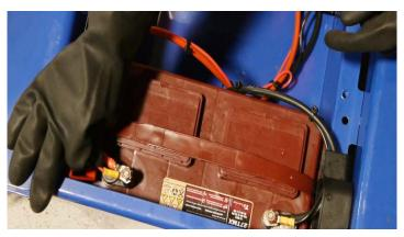
Using a hydrometer, check the specific gravity of each cell in the battery. The hydrometer should read between 1.28 and 1.285, and all cells should be equal.
