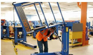
Lower the cage and undo the two main fixing bolts. With the sling or hoist, remove the complete cage. (This has been demonstrated on a Nano same procedure for Nano Sp.)
