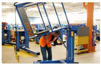
Place some oil soak cloths around the power pack pipe connection and undo the pipe connection. Locate the spine cap and remove, loosen the pipe, there may be a small amount of oil spillage. Locate the two power pack fixing screws,
