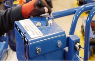
Remove the additional load, leaving the 200 kilograms in the platform, and elevate the machine to full height from the ground controls to ensure the alarm does not operate prematurely
