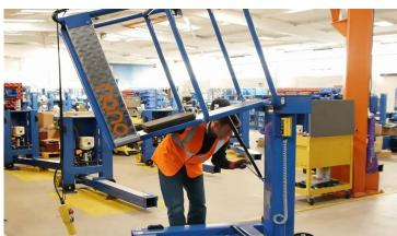
Lower the cage and undo the two main fixing bolts. With the sling or hoist, remove the complete cage.
