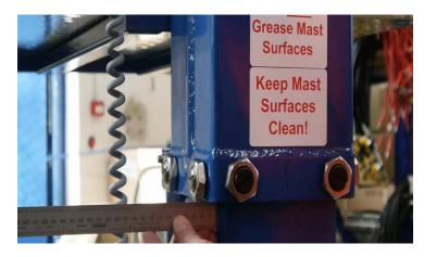
Screw in the four side wear screws, so that they just make contact with the 0.2 feeder gauge, slightly back if the gauge cannot be withdrawn, and tighten the lock nut. Repeat the process for the middle mast section to lower the mast.
