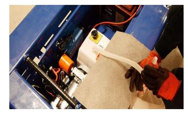
Refill with 4.5 litres of grade 32 mineral oil. Elevate the machine from the ground controls to ensure the platform reaches full travel. If not add a little more oil. Do not keep the pump running with no oil in the tank.
