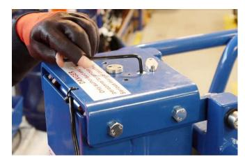
Elevate the platform to approximately two metres so that the second mast section is lifted approximately 400 millimetres.
