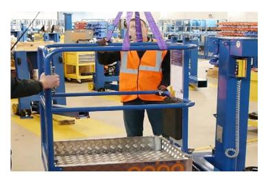
Remove the tool tray on top of the mast. Undo the four bolts surrounding the mast cap and operate the lift function from the ground controls so that the mast caps complete with spring assembly, clears the mast section.
