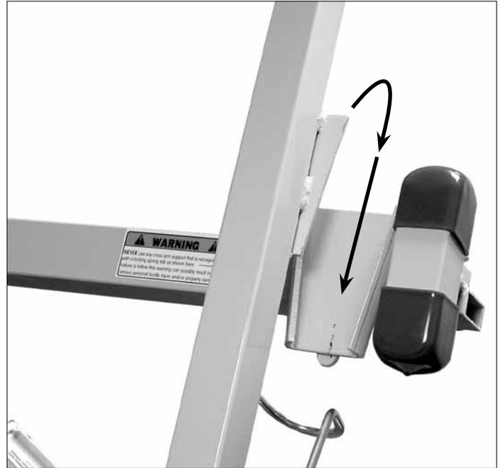
9. Place the tapered plates of the cross arms into the tapered sockets on the cradle. The spring tab on the back of the cross arm will lock it into place.
