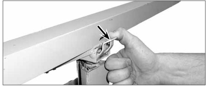
8. Mount the cradle on top of the telescoping section. Flip out the tilt latch to allow the cradle to tilt for loading and for hanging drywall on sidewalls and sloped ceilings.
