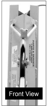
10. To reinstall the assembled telescoping sections, feed the crimped end of the cable through the frame sheave pocket from the top and over the top of the sheave as shown.
