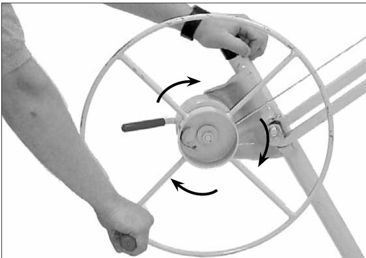
13. Rotate the winch in the direction shown to take the slack out of the cable.
