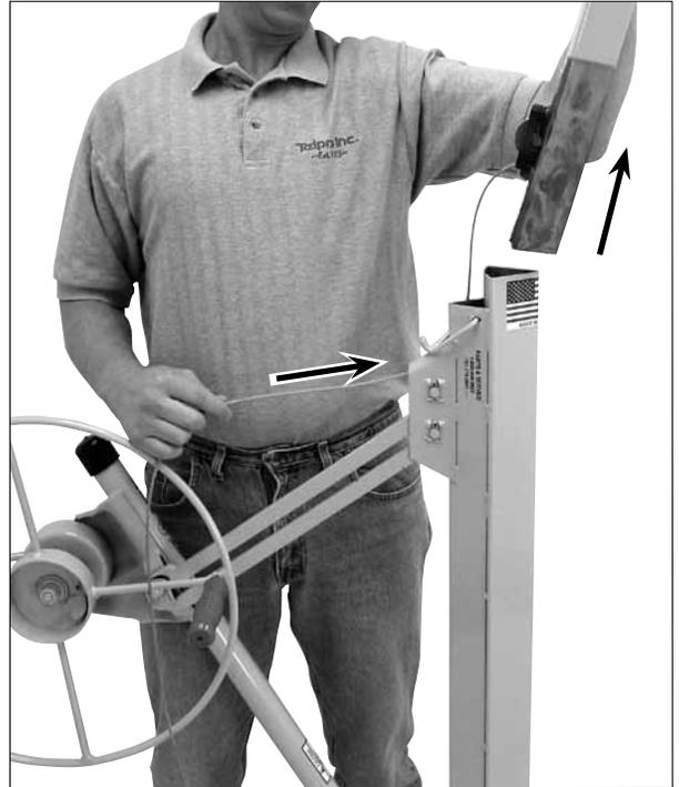
3. Remove the two telescoping sections completely from the frame housing. Pull the cable completely out from the frame along with them. **BE CAREFUL** for loose strands or frays on the cable.
