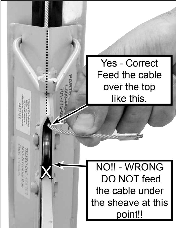
5. MAKE SURE that the cable feeds over the TOP of the cable sheave as shown in the above photo.
