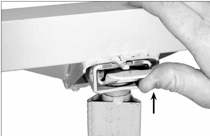
3. Lock the cradle tilt latch and lift the cradle off of the frame.
