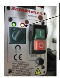
Indicator turns orange when too much pressure is added on the cutter. Will turn Red and cut power to motor if machine is given too much force for the motor to cope with.
