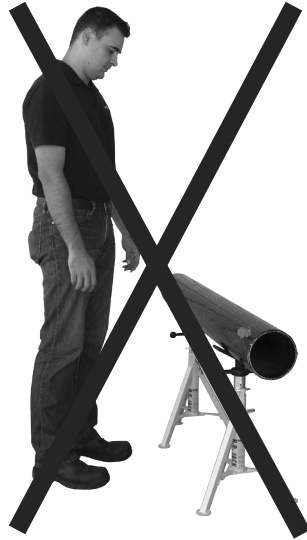
Incorrect Jack Height Work too low for operator can result in back injury.
