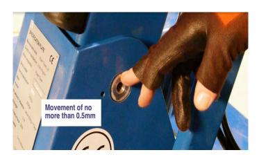
If the movement is above the tolerance, then replace the pin use a small amount of Loctite 648 when replacing the plastic pin caps
