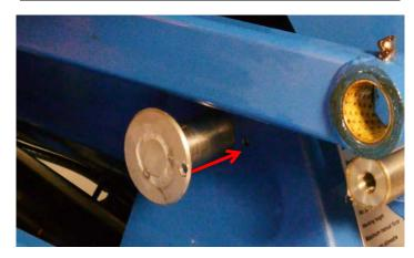
Replace the M6 pivot locking screw. Ensure to use a small amount of thread lock 648 on M6
