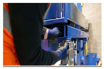
Refitting is a reverse of this procedure but it is essential to fit a spacer washer but when tightening the fixing bolt, ensure it is torque to 55Nm, ensure the wheel moves freely.
