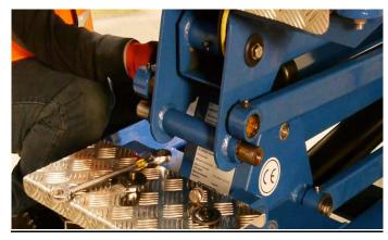
Then remove the M6 pivot locking screw and use a suitable rod (diameter 30 millimetres), or another pin, to push out the old pin.
