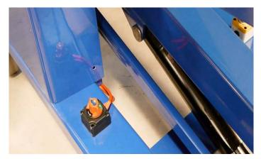
Check the battery charger lights when first switched on (Display Green LED On, Amber LED blinking fast is bulk load, blinking slow is absorption, on float, off storage.) If the both charger lights flash slowly, check the fuse, battery connections and then the battery condition as outlined in the chapter: 'Battery Maintenance'.
