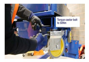
Ensure the wheel spins freely and rotates on the castor if the wheel doesn't move freely after being tightened to the required torque then fit a spacer washer. Check for any damage, the breaking latch moves freely and the castor is not twisted.
