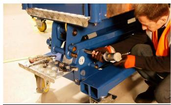
With a new pin (part Number PT- M- 120 OR 120S), align the hole on the pin with the hole on the chassis. And tap into place with a mallet.
