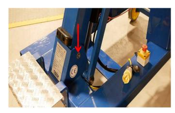
Stand by the side of the machine and push the boom, just above the middle knuckle post, sideways, back and forth.
