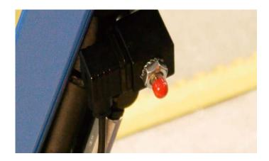
Remove the red cap. Identify the direction of the bend and, using a pair of pliers, gently straighten the bend.
