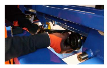
Replace in the reverse sequence. Apply a small amount of Loctite 648 when replacing the M12 bolts.
