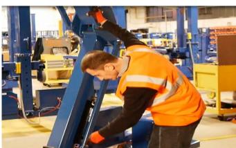
Observe the end of the lower boom to chassis pivot pin and see if there is any movement on the hole.
