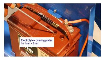
Check the connections and make sure the battery is clean
