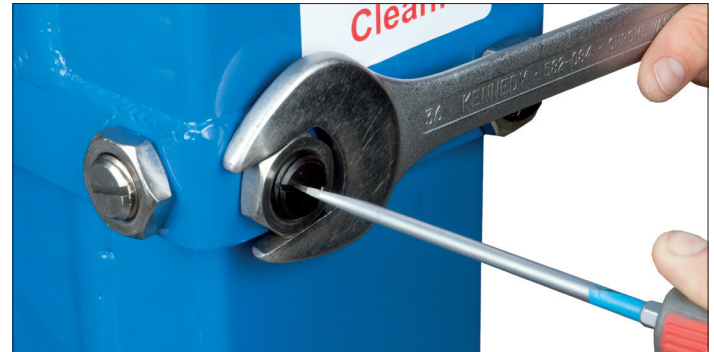
Mast wear screw adjustment
