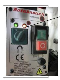
Indicator turns orange when too much pressure is added on the cutter. Will turn Red and cut power to motor if machine is given too much force for the motor to cope with.
