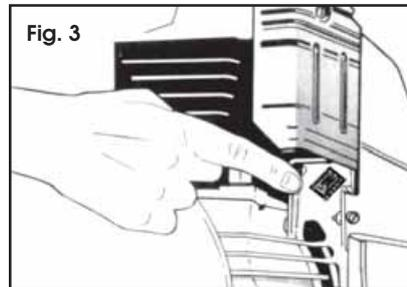
b. The motor is protected by a Thermal Overload so that if the motor overheats for any reason - the thermal overload will trip, stopping the motor. To restart, allow a period for the motor to cool down, before pressing the Reset Button, shown in Fig.3.
