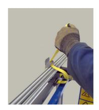
Each jaw bracket has a simple, yet highly effective, lashing strap that can either gather and bundle loose materials and tubing, or restrain larger single items such as ducting/beams etc. The hard wearing shock absorbing pads reduce slip and prevent damage to any materials carried.
