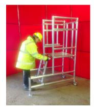
5) CLIP UPPER BRACE OF LADDER ABOVE RINGS ON VERTICALS WITH ASSEM-BLED HOOKS AT TOP
