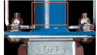
4. Apply an even amount of copper slip around the castor with a small paint brush; this will enable you to apply the lubricant around, up and behind the plastic collar.
