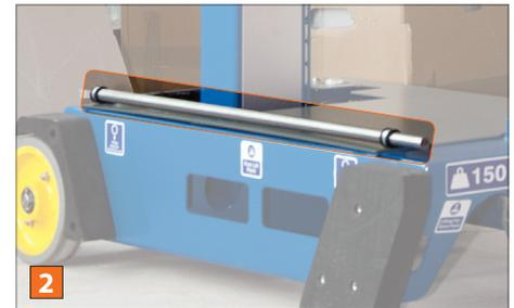
Emergency lowering tool located on chassis
