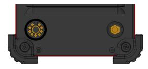
**Torch Connector:** Connect here the cutting torch. The torch connection to the power source is very easily performed through a quickconnector carrying the torch trigger circuit, the gas line and the torch power cable.
