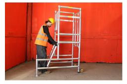
4) CLIP UPPER BRACE OF LADDER ABOVE RINGS ON VERTICALS WITH ASSEMBLED HOOKS AT TOP
