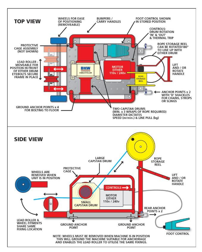
BEFORE ANY OPERATION USING CABLE-PULLER, THE UNIT MUST BE SECURELY ANCHORED. FAILURE TO DO SO MAY RESULT IN PERSONAL INJURY AND DAMAGE TO THE MACHINE.
