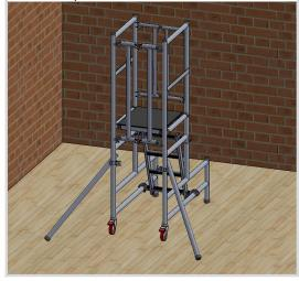
stabilisers at 90° from the Podium, and 1 parallel to the wall
