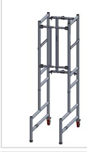
3. Ensure the bottom locking elbow has engaged.
